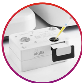
Insert Sample in the Cartridge
